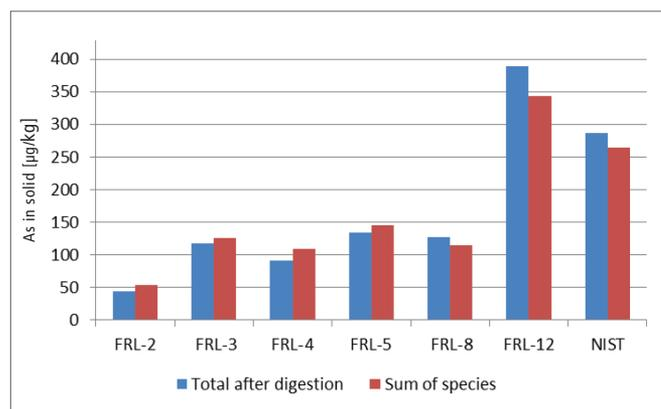
Figure 4. Comparison of sum of species obtained by LC-ICP-MS with totals obtained after microwave digestion.
