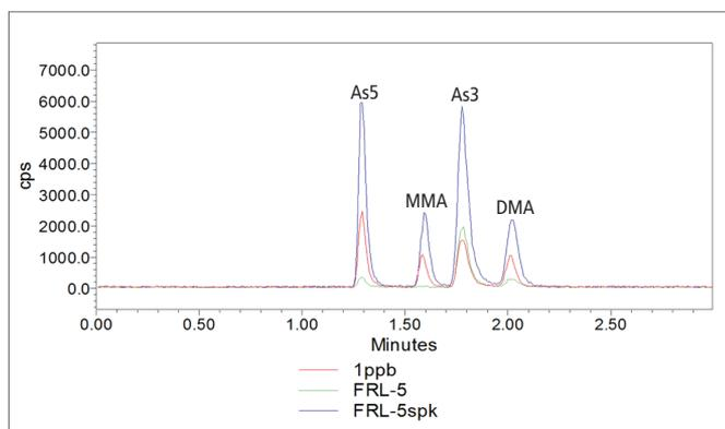
Figure 1. Separation of arsenic species achieved using ion interaction chromatography. Overlay of 1 ppb standard in mobile phase, and FRL-5 sample extract (brown rice flour) with and without 2 ppb spike.
